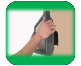
2. Mount the system onto the bracket
