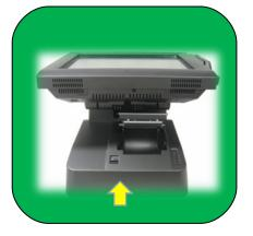
2. Push the lever to open the printer cover.
