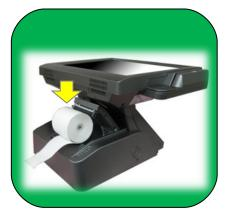
3. Replace paper roll, and pull paper to extend outside the printer.
